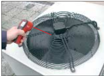
Safely diagnosing the status of a system by measuring the temperature of safety valves, pumps and other wearing parts.
